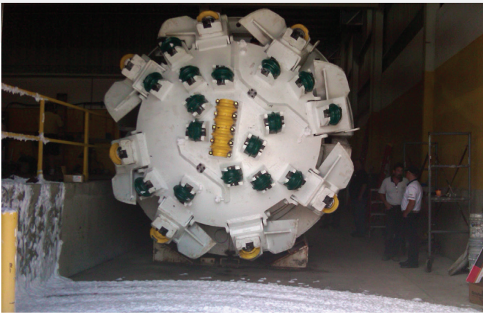
This large boring device was used to help build the $110 million Western Regional Conveyance Tunnel. The 32,610-foot tunnel routes flow to the Western Regional treatment plant. It was recognized as the Environmental Initiative of the Year by New Civil Engineer magazine in 2013.
